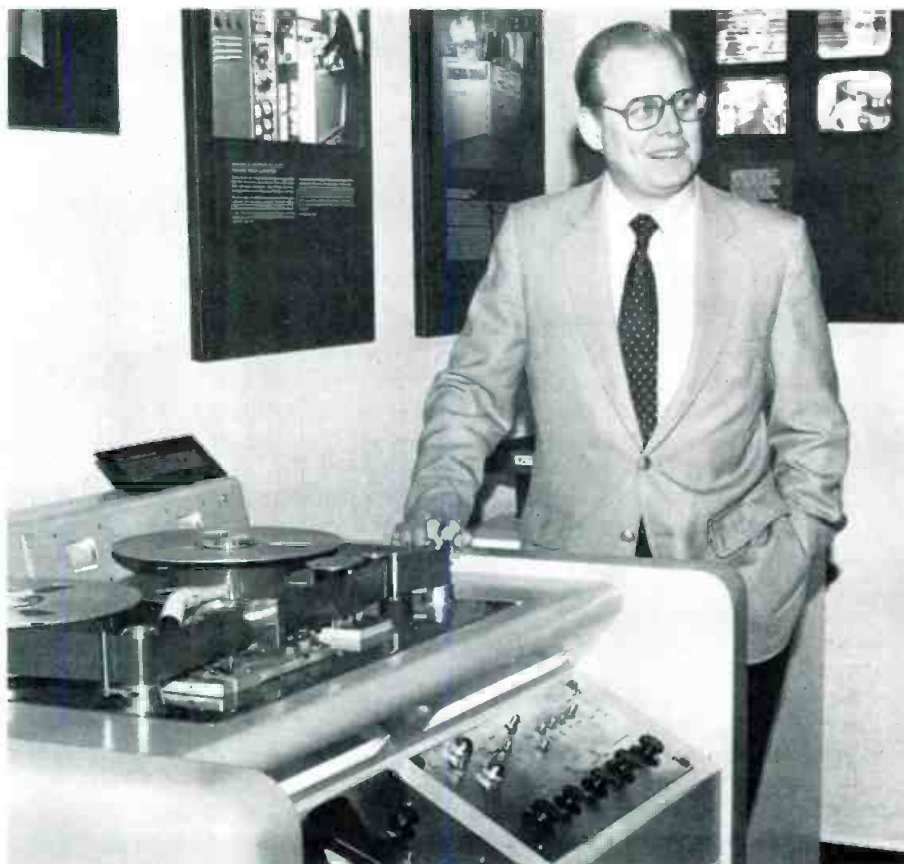
Peter Hammar, curator of the Ampex Museum of Magnetic Recording, shows off one of the centrepieces of the museum, an Ampex VRX-1000 video tape recorder. This one was the fourth one produced by Ampex and the first delivered to a customer, the CBS Television Network, in 1956.
